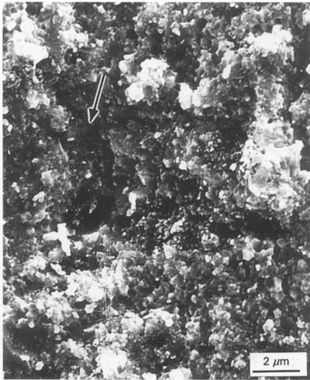
Figure 5 Fracture origin in a 20 vol % SiC w /TZP composite showing the SiC fine-particle clustering (arrowed).
